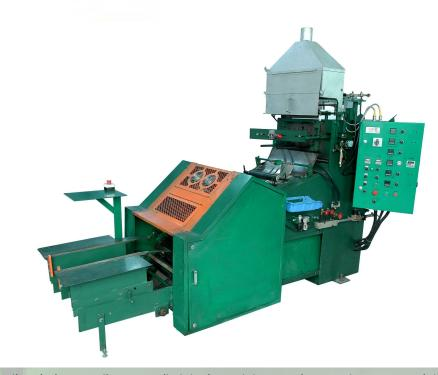
power fed in and out of trim die. (Die cooling available.) Mold spraying systems provide clean filtered air free of oil and water for both mold spray gun and vent bars. Individual air cylinders are provided for both mold opening/closing and for grid ejection. Lead valve and lead dispensing ladle are gas purged to reduce dross. Simplified cast grid slow down system to minimize grid distortion. Maximum cast grid thickness .150 in.(3.9mm) x 158.75mm Trim Width x 385.75mm Lug to Lug.
